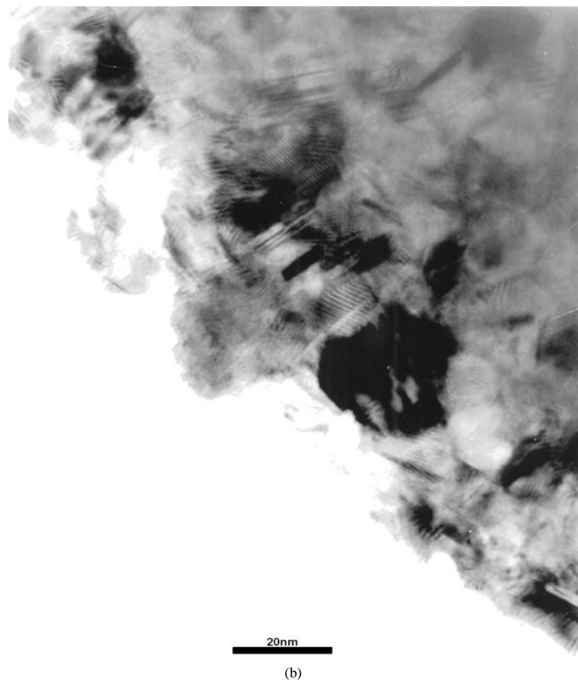
Figure 5 (a) Bright field TEM image of a CuO grain reduced to Cu and ED pattern taken from the entire grain. (b) Section of (a).
